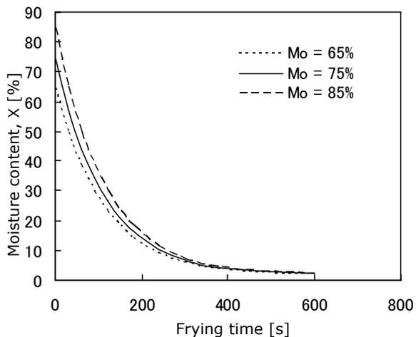
**Figure 2.** Effect of initial moisture content for oil temperature 118°C and vacuum pressure 9.89 kPa
