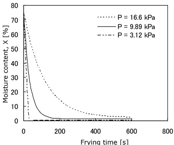
**Figure 3.** Effect of vacuum pressure for oil temperature 118°C and initial moisture content 75%
