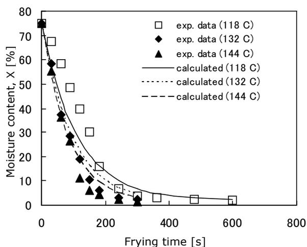
**Figure 1.** Moisture content as function of frying time for various oil temperatures at vacuum pressure 9.88 kPa.
