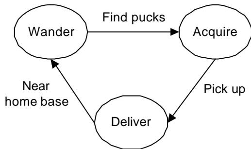
Figure 3: The behavioral states of the robots
