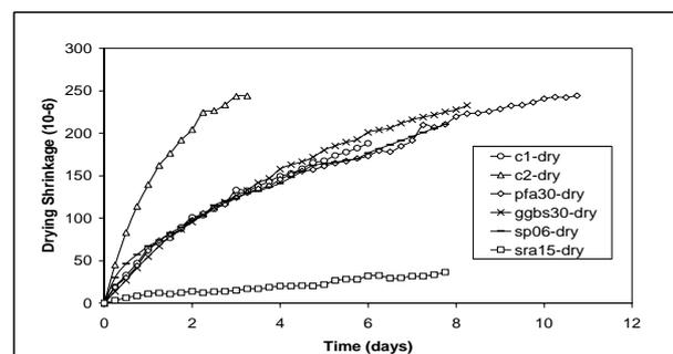
Figure 17. Drying Shrinkage of All Mixes Observed in The Current Research
