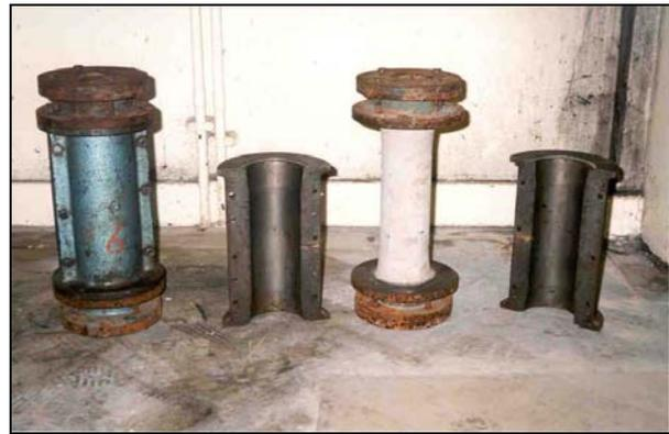
**Figure 1.** An example of bobbin shaped specimen where it was cast in the bobbin-shaped mould (left) and after concrete hardened the middle sections of the mould were removed leaving the specimen with end caps (second from right).
