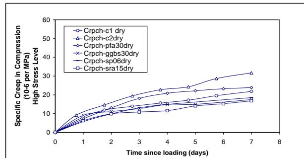
Figure 10. Total Compressive Creep (High Stress) Determined on Drying Specimens
