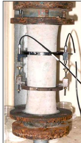
Figure 4. Arrangement of LVDTs on The Specimen
