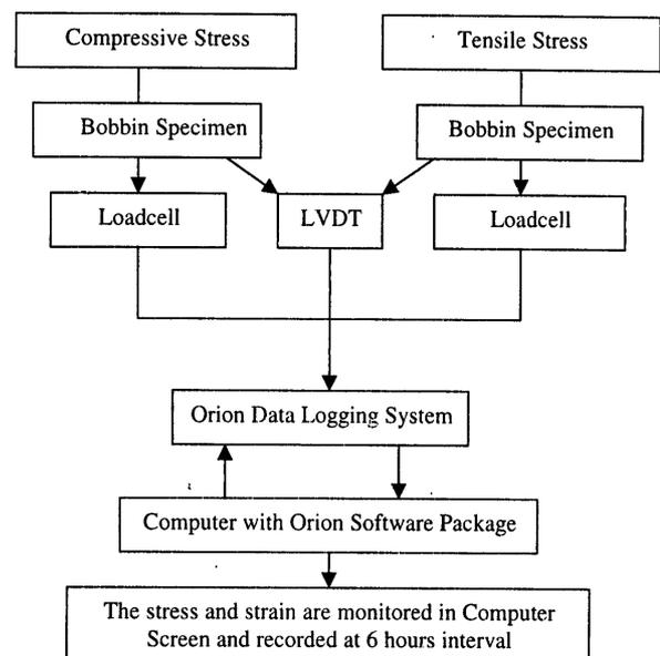
Figure 5. The Scheme of Data Acquisition System
