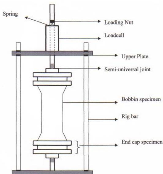
Figure 3. Tensile Creep Test Frame
