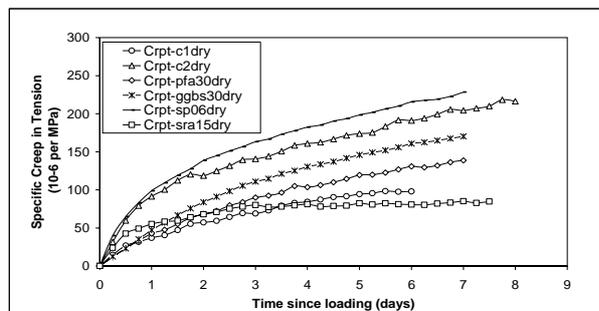
Figure 8. Total Tensile Creep of Concrete Determined on Drying Specimens
