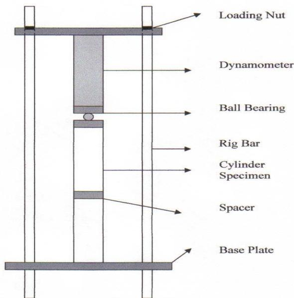
Figure 6. Compressive Creep Loading Frame (High Stress Level)
