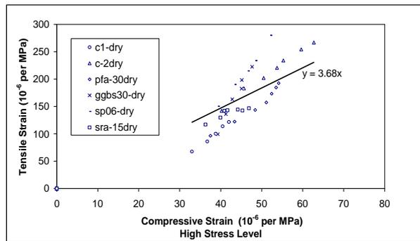
Figure 14. Relationship Between Creep Function in Tension and Compression Based on Equal Applied Stress/Strength Ratio.
