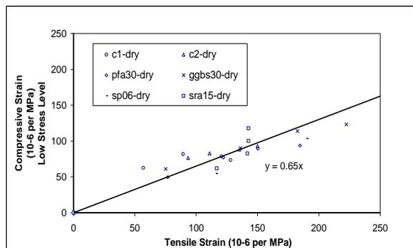
Figure 12. Relationship Between Creep Function in Tension and Compression Based on Equal Applied Stress.
