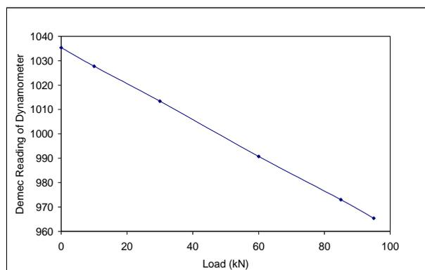
Figure 7. Example of The Result of Dynamometer Calibration.
