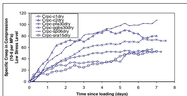
Figure 9. Total Compressive Creep (Low Stress) of Concrete Determined on Drying Specimens.
