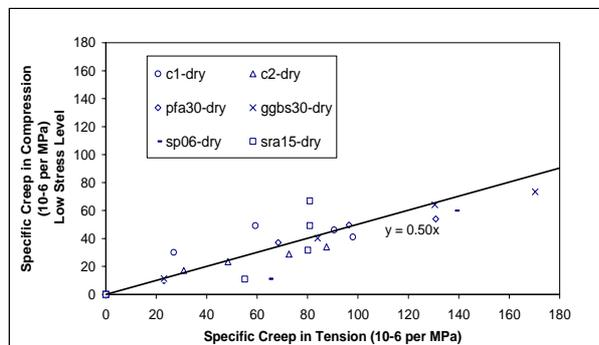
Figure 11. Relationship Between Specific Creep in Tension and Compression Based on Equal Applied Stress.
