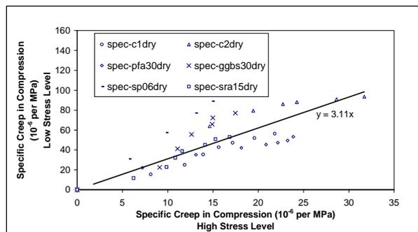
Figure 15. Relationship Between Specific Creep in Tension Determined From Low Applied Stress and High Applied Stress Level.
