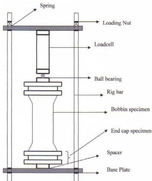
Figure 2. Compressive Creep Test Frame
