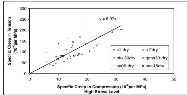
Figure 13. Relationship Between Specific Creep in Tension and Compression Based on Equal Applied Stress/Strength Ratio.
