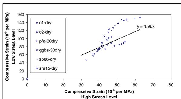
Figure 16. Relationship Between Creep Function in Tension Determined From Low Applied Stress and High Applied Stress Level.
